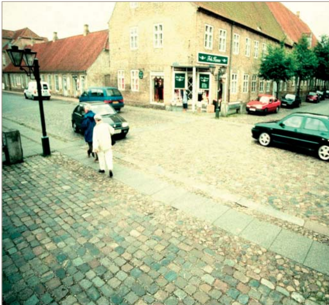
Fig. 10. Fatalities and serious accidents ceased and traffic tailbacks reduced when all traffic signals, signs and road markings were removed from the central junction in Christiansfeld, Denmark
